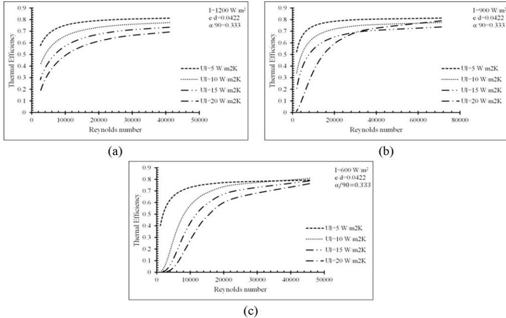
**Figure 2:** variation of thermal efficiency with Reynolds number at different levels of heat loss coefficient.
