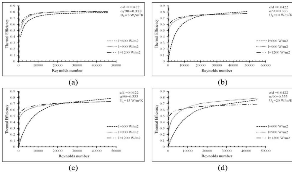
**Figure 1:** variations of thermal efficiency with Reynolds number at different levels of solar Insolation.
