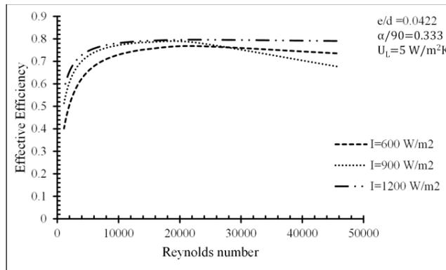
**Figure 3:** variation of the effective efficiency with Reynolds number.
