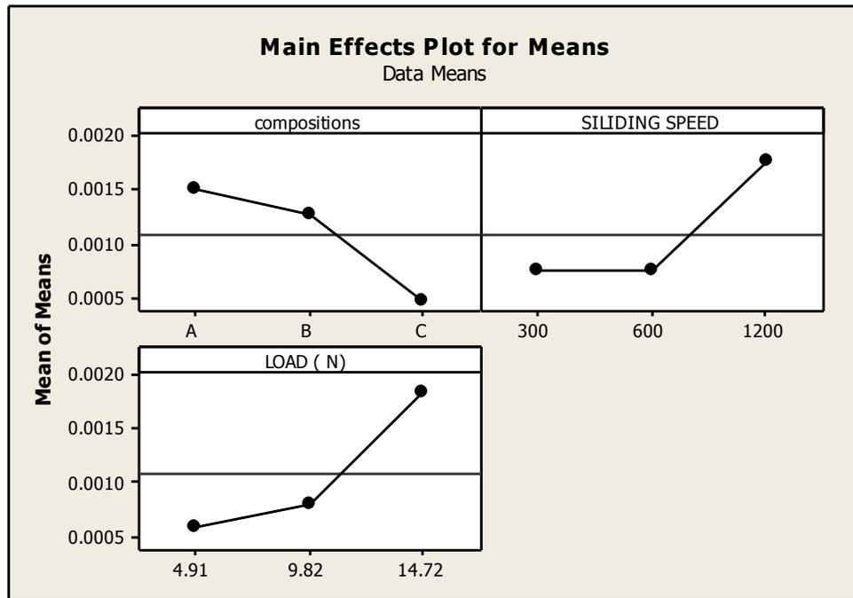
Figure 2: Showing the effect of load (N), composition and sliding speed (rpm) on mean wear rate
