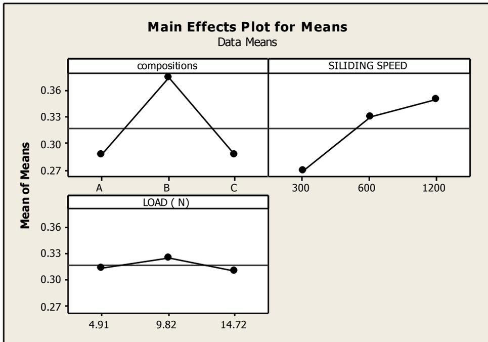
Figure 3: Showing the effect of load (N), composition and sliding speed (rpm) on mean of coefficient of friction
