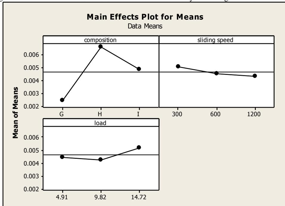
**Figure 4:** Showing the effect of load (N), composition and sliding speed (rpm) on mean wear rate
