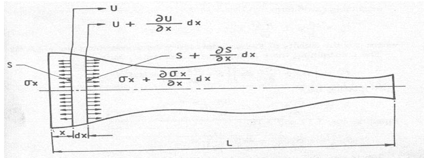
Fig. 1 Scheme of free-free vibration of non-uniform bar [7].
