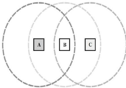
Figure 1.1: A Mobile Ad hoc network of nodes, where nodes A and C must determine the route through B in order to communicate.
