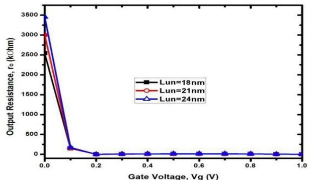
Fig. 8 compares the output resistance of the three devices. Greater the underlap, greater is the output resistance. Thus, the device with 18 nm underlap shows minimum  $r_o$ , the device
