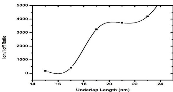
Fig. 6. Variation of Ion/Ioff ratio of A-U-DG-GS MOSHEMT for various underlap lengths.
