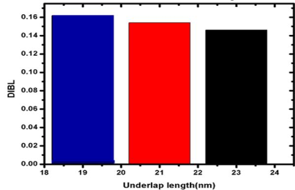
Fig. 7. DIBL for various underlap lengths of A-U-DG-GS MOSHEMT at  $V_{ds} = 0.5$  V and  $V_{gs} = 1$  V.
