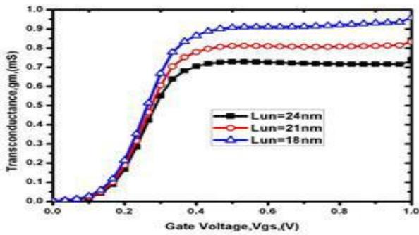
Fig. 4. Comparison of gm of A-U-DG-GS MOSHEMT with various underlap lengths as a function of  $V_{gs}$ , at  $V_{ds} = 0.5$  V.
