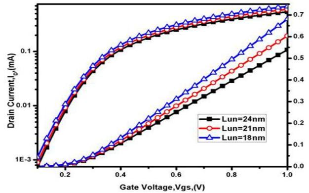
Fig. 2. Comparison of Id of A-U-DG-GS MOSHEMT with various underlap lengths as a function of Vgs, at Vds = 0.5 V the device with 21 nm underlap shows lower on current and the device with 24 nm underlap shows the least on current.
