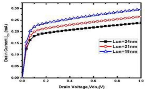
Fig. 3: Comparison of Id of A-U-DG-GS MOSFET with various underlap lengths as a function of Vgs, at Vds = 0.5 V.
