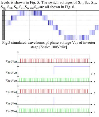
Fig.6. Simulated waveforms of switch voltage for inverter stage with in a line period [Scale: 100V/div]
