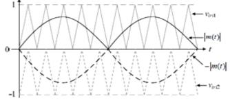
Fig.4 Modulation strategy: carrier/reference signals
