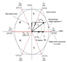
Fig.9. Inverter output voltage space vector
