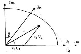
Fig.9.3 Definition of the Space vector Depending on the switching times t0, t1 and t2 the space
