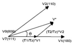
Fig 9.1 Determination of Switching times
