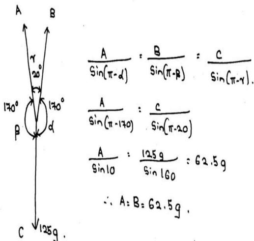
Fig. 5. Lami's theorem and geometry of load application
