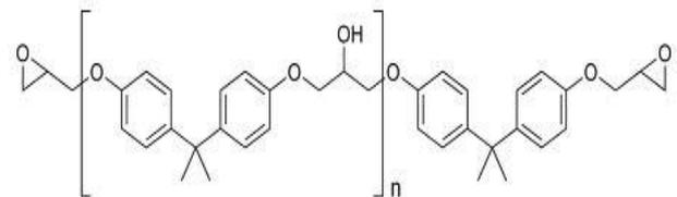
Fig. 1. The typical structure of epoxy
