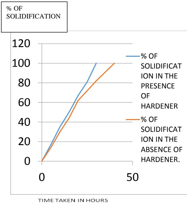
Fig. 7. Time taken for composite formation with and without hardener(i.e. time taken for the solidification of epoxy with and without hardener)
