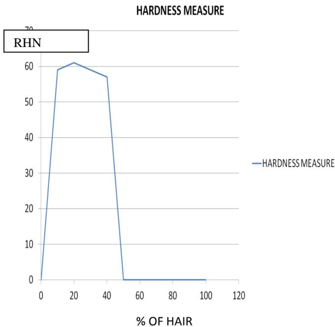
Fig. 10. Comparison between % of hair and rockwell harness number
