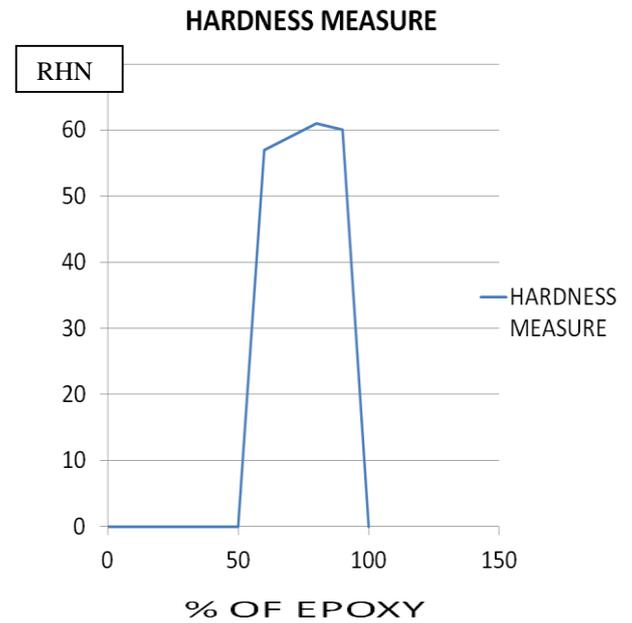
Fig. 8. Comparison between % of epoxy and rockwell harness number
