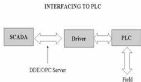
*C. Input-Output Configuration for PLC*
