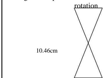
Fig. 2. Shows the area swept by the rotor of the model while rotation. In HAWTs, the shape of swept area is defined by rotor radius.
