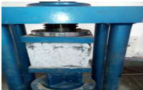
Figure 3 cube under compression testing machine (CTM)
