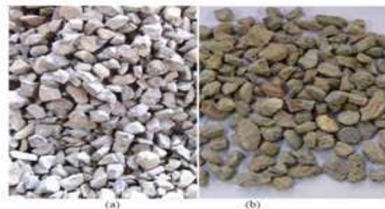
Figure 1 Texture comparison between Natural aggregate & Recycle aggregate
