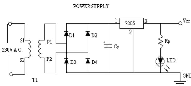
Step-down transformer is used to convert the 230v AC into 12v AC as required to the project. The power supplies used in our project are +5V and +12V. Rectifier is used to flow the current only in one direction. It is used in power supply operation. It can carry higher current than other diodes[5]. Voltage regulator is used to control the unregulated power supply. ADC and DAC is used for conversion of voltage.
