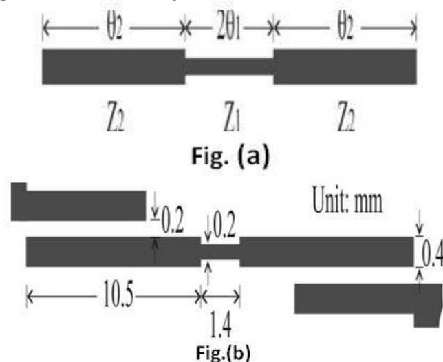
Fig. 1 Geometrical diagrams of the stepped-impedance resonator (SIR) and its constituted dual-band bandpass filter. (a) SIR ( $RZ < 1$ ); (b) one-stage SIR bandpass filter (coupling length:  $LC1$ ).
