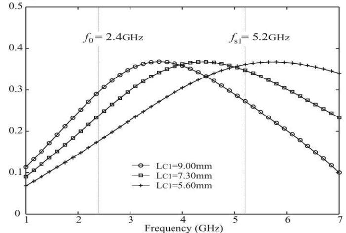
Fig. 3(a) and Fig. 3(b) illustrate the derived normalized J inverter susceptance ( $J$ ) and equivalent electrical length ( $\theta/2$ ) under different lengths ( $LC1$ ). The parameter  $J$  is seen to increase, reach to the maxima and then decrease as a nonmonotonic function of the frequency over 1.0 to 7.0 GHz for all the three cases. Further, as the length ( $LC1$ ) is stretched, the band and stronger at the second operating band. In other words, the FBWs of both bands may be freely
