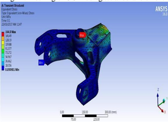
Fig.12. Von Misses Stresses on Upper Control Arm
