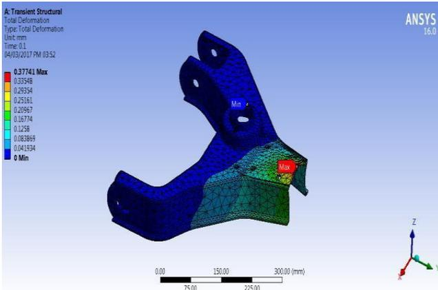
Fig.8. Deformation of Upper Control Arm
