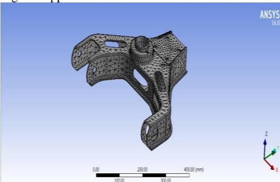
Fig.11. Meshing of UCM using tetrahedral element
