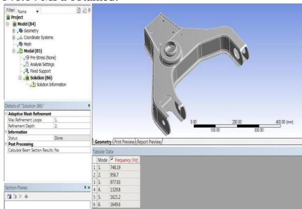
Fig.9. Natural Frequency of Upper Control Arm
