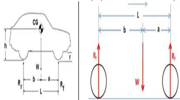
Fig.1. Forces on Stationary Car
