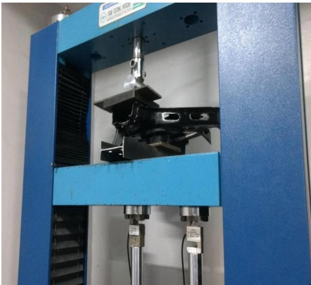
Fig.14. Testing of Arm on UTM
