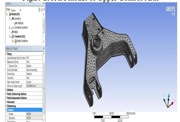
Fig.6. Meshing of Upper Control Arm using Tetrahedral Element
