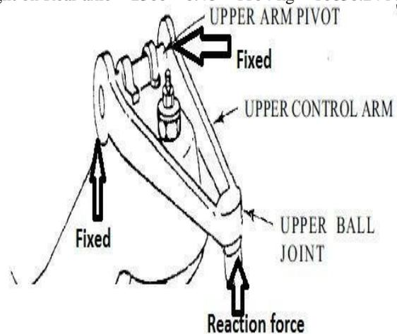
Fig.2. Boundary forces for Static Condition
