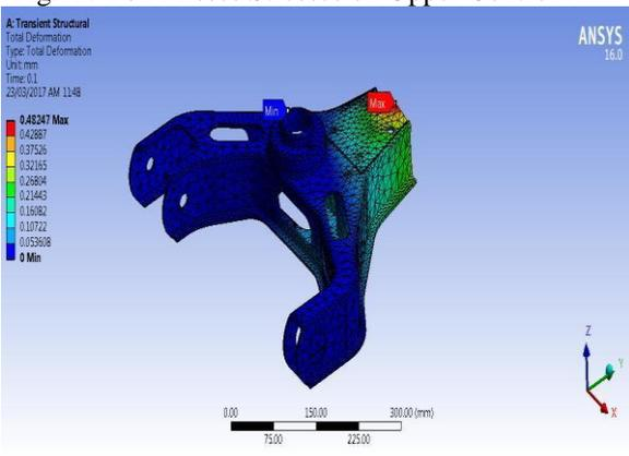
Fig.13. Deformation of Upper Control Arm
