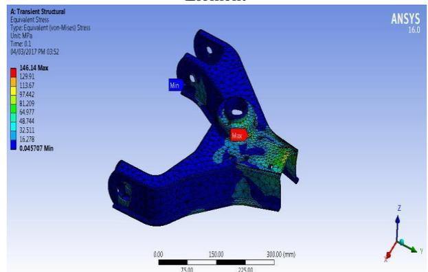
Fig.7. Von Misses Stresses on Upper Control Arm
