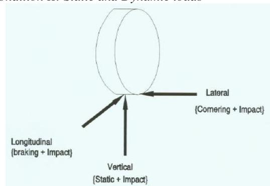
Fig.3. Wheel Loads and Directions
