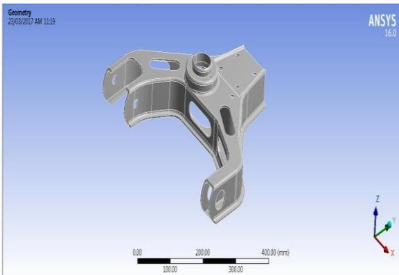
Fig.10. Upper Control Arm with Profile Modification
