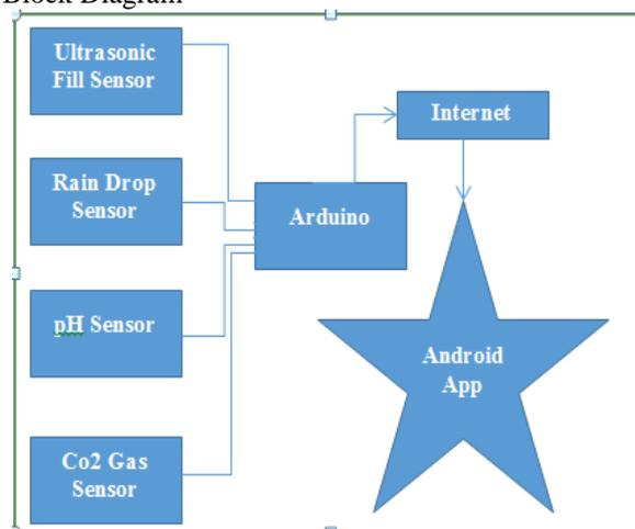
Ultrasonic fill sensor: To measure the level of waste in the smart bin we used ultrasonic sensor attached in the top of the bin. The ultrasonic sensor is providing ranging measurements independently of the contained objects, thus making possible the corresponding translation into fill level measurements. Moreover, ultrasonic sensors are most suitable to this application because they can be placed on the lid and thus avoiding harsh conditions of the
