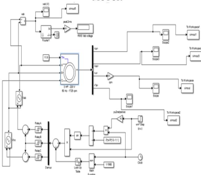
Fig 1. Matlab Model of Induction Motor
