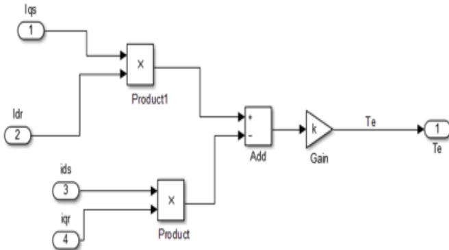
Fig 3. Torque Equation based on Flux linkage
