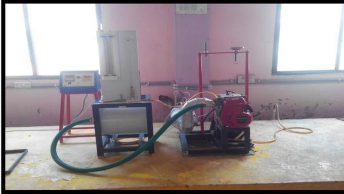
Fig.3.2 Single cylinder for stroke petrol engine with rope brake Dynamometer
