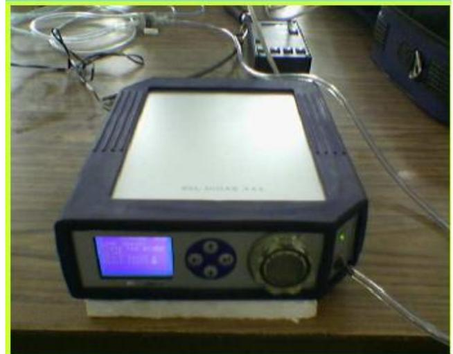
Fig. 3.3 AVL DIGAS 444 Gas Analyzer
