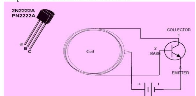
Fig. 3 Wireless Power Transfer Circuit
