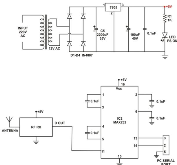
Fig. 11 Circuit diagram of central receiver hub
