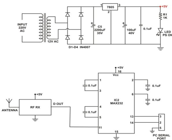
Fig. 6 Circuit Diagram of central receiver hub
