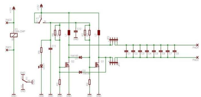
Figure 7 Wireless power transmitter circuit
