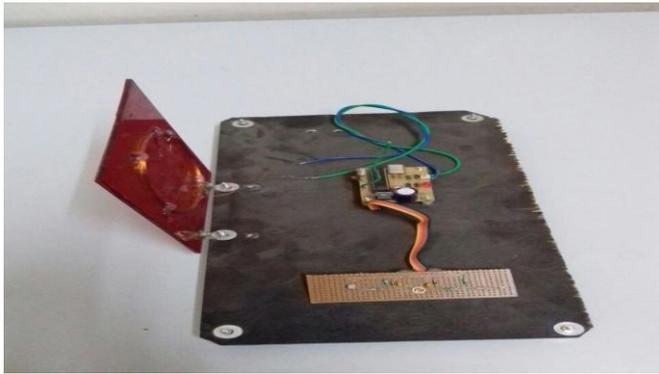
Fig .10 Hardware implemented Wireless Sensor Node
