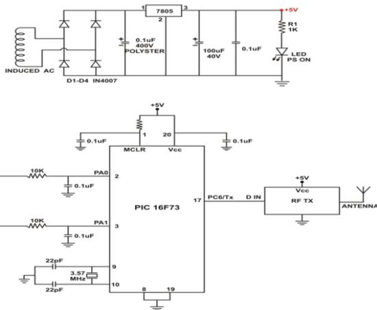
Figure 5 Energy harvesting wireless sensor node (Receiver)
