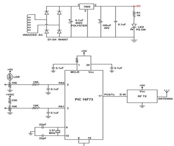
Fig. 9 Wireless sensor node (receiver)
