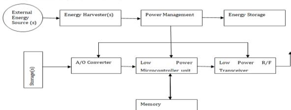
Fig 1. System architecture of a wireless node with energy harvesters
