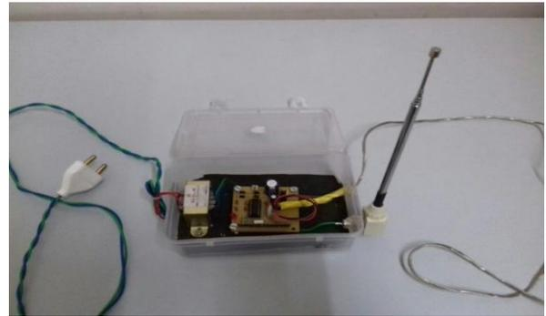
Fig. 12 Hardware implemented Central Hub
