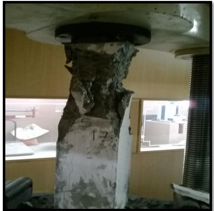
Fig ...Failure pattern of column due to compressive load
