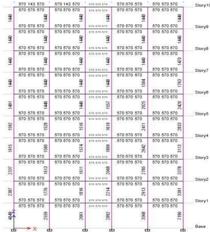
Figure: Reinforcement required for 30.5m model after considering mass eccentricity (Outer face)
