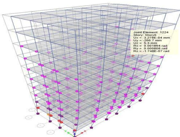
Figure. Pushover Analysis of Asy2 Structure.(8th Time step)
