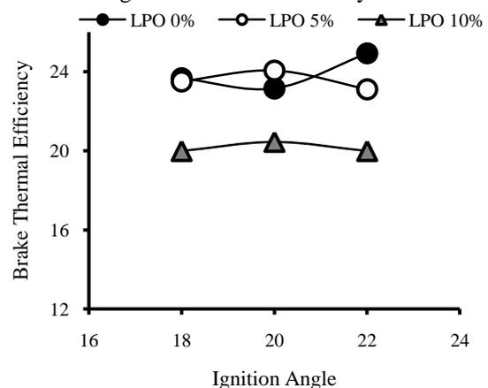
Figure: 1 Variation of Break thermal efficiency with ignition angle for different blends
