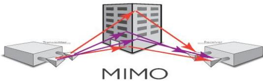
Fig1: MIMO exploits multipath propagation to multiply link capacity[9]
