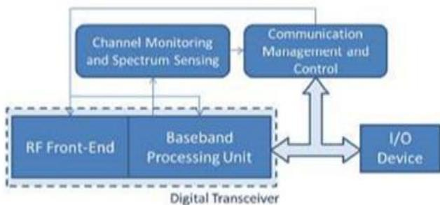
Fig 2: cognitive radio physical architecture.[8]
